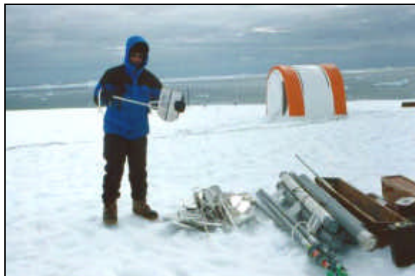
In 1994, Ralph, KØIR holds one of the snow anchors used to secure the antennas and shelters.
